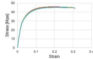
Stress/Strain curves for ISO 527 specimens, PBF2.
