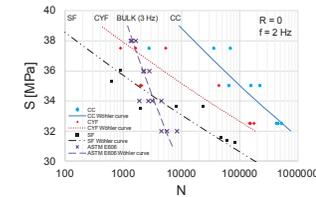
Wöhler curves for lattice and ASTM E606 specimens, PBF1.
