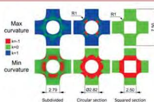
Curvature analysis of unit cells.
