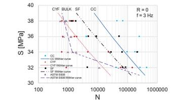
Wöhler curves for lattice and ASTM E606 specimens, PBF2.
