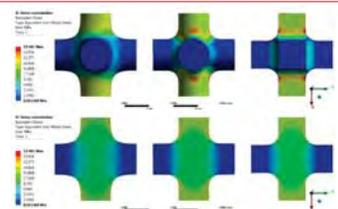
Stress distribution analysis of unit cells (full cell above, sectional view below).
