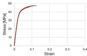
Stress/Strain curves for ISO 527 specimens, PBF1.
